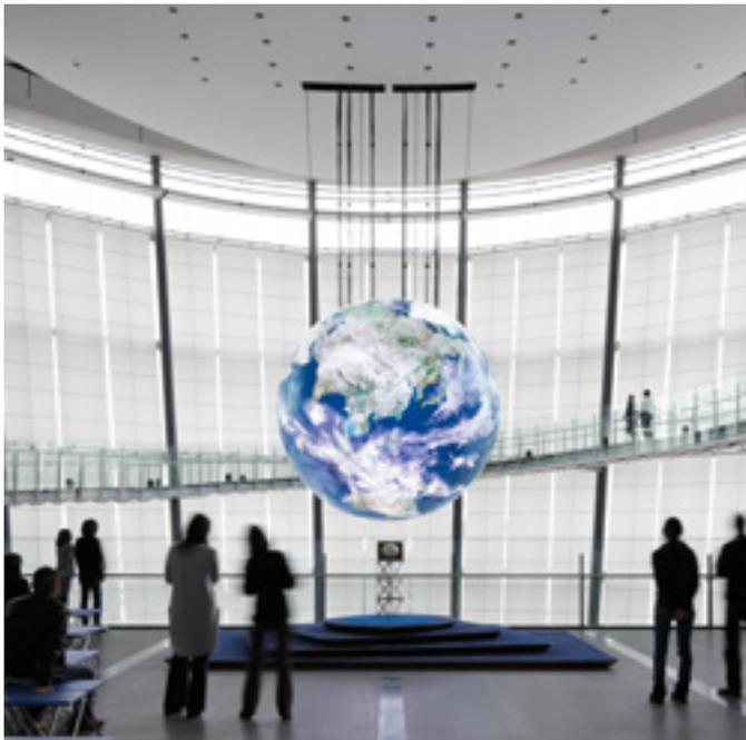
Luminescence device: Organic LED (10,362 square panels (96 mm)). Size: Diameter 6 meters (Approx. 1/2 millionth the size of the Earth). Number of pixels: 10 million pixels and over. Inner structure: Geodesic octahedral model
